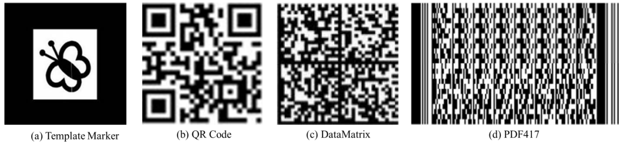
Fig. 3. Illustration of 2D markers. (a) Template marker. (b)-(d) Barcode markers: QR code, DadaMatrix and PDF417.
