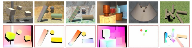
Fig. 2. Ground-truth optical flow data. The top row depicts some example images from our system. Below is the ground-truth flow between successive frames. The flow field color is coded using the same format as [1]. Black values in the flow image indicate areas of occlusion between the two frames.
