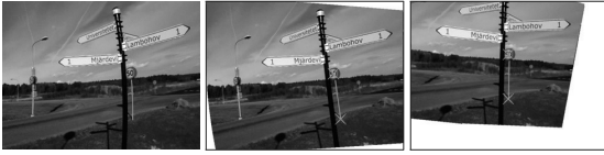
Figure 11. Image stabilisation. Left: Uncorrected RS frame. Centre: Rectified frame, with tracked points indicated. Right: Frame stabilised by centring the tracked points along a vertical line.
