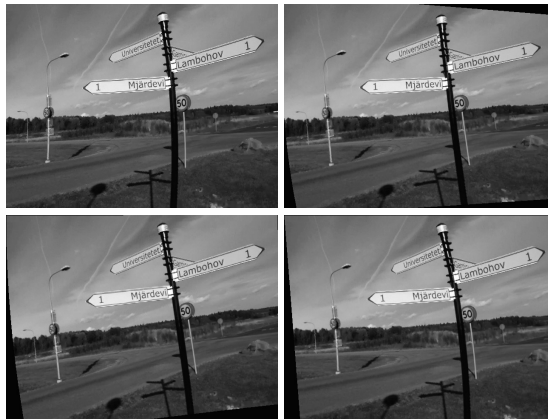
Figure 1. Example of rolling shutter imagery. Top left: Frame from an iPhone 3GS camera sequence acquired during fast motion. Top right: Rectification using our rotation method. Bottom left: Rectification using the global affine method. Bottom right: Rectification using the global shift method. Videos are available on the web and in the supplementary material.
